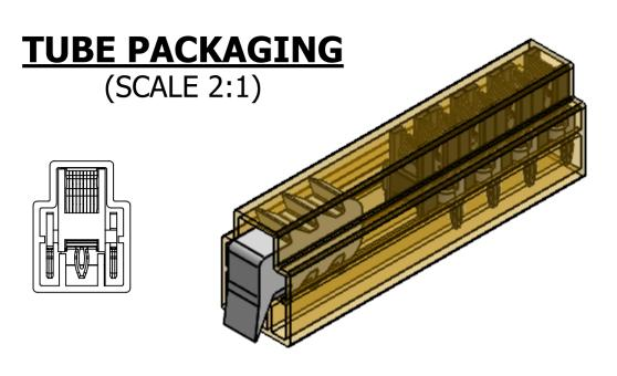
TUBE LENGTH: 340mm (13.4") TUBE WIDTH: 12mm TUBE HEIGHT: 16mm QTY PER TUBE: 50 PCS
